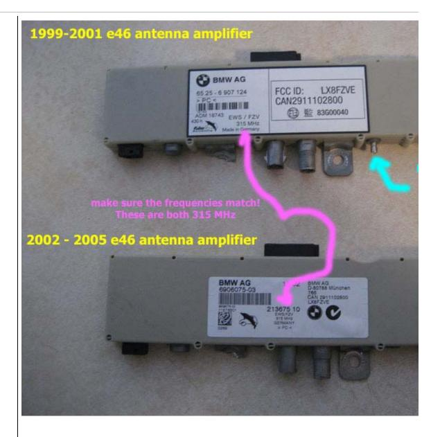
Once you have ordered the proper antenna amplifier (circa \$200 from the dealership), insta flat head screwdriver and a T20 torx screw driver as well. If you can find a stubby T20 torx, to unscrew.
