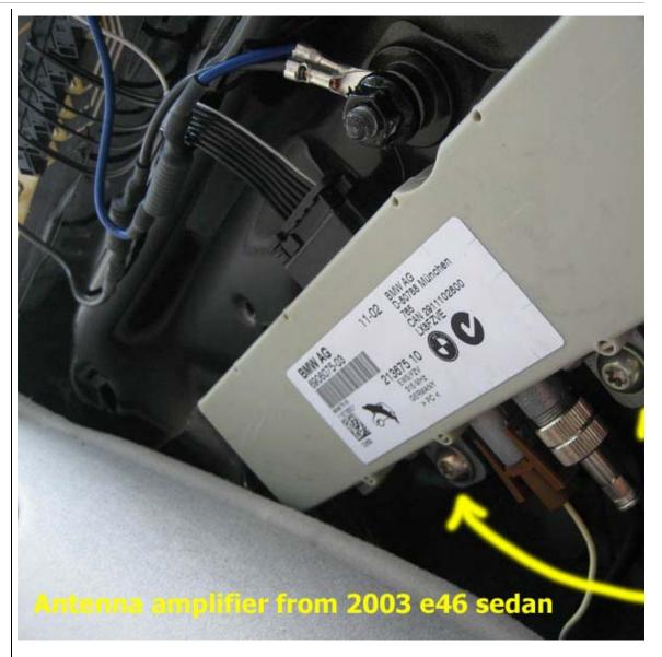
**Step 4:** Connect the new antenna amplifier. I found it easiest to connect all the wires first, there is an extra wire now (this is the wire that powered the older style amplifier that termindeck. This wire is now connected to nothing at both ends.
