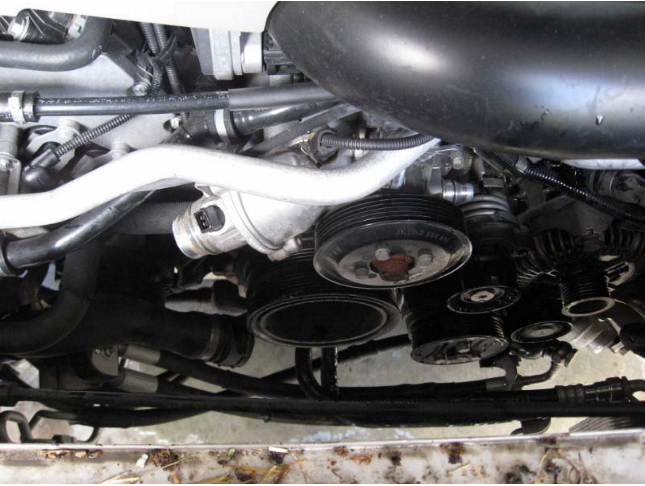
Removed water pump pulley.
