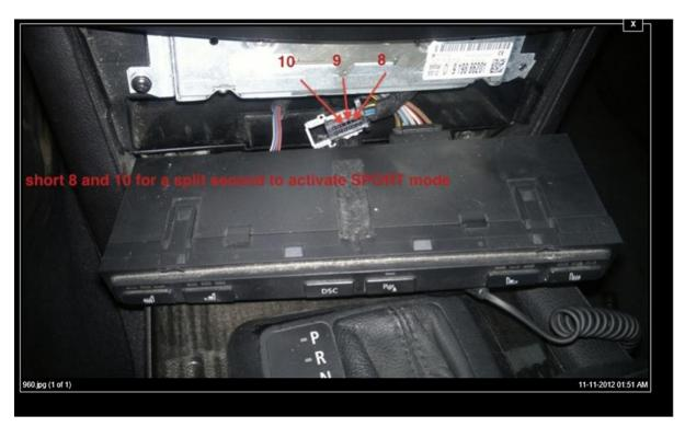
Pins 1 - 9 Button LED Pins 2 - 10 Button ground Pins 3 - 8 Button live
