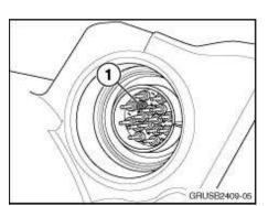
5. In some cases, the incorrectly installed sealing sleeve may permanently damage pins in the Mechatronic connector (X8500). In such a case, the Mechatronic module has to be replaced (**pin repair is not possible**). The illustration shows an example of a broken and missing pin #4 in the X8500, caused by improper sleeve installation; this resulted in the customer's complaint about the inoperative Sport Mode of the transmission.
