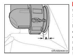
4. If the distance between the connector and the transmission housing (A) measures approximately 7 to 8 mm, the sealing sleeve was installed incorrectly. In such a case, an intermittent connection problem between Mechatronic and the vehicle harness connector will occur, resulting in various EGS communication faults (e.g., FC 5079 "Serial wire message missing"; FC 507A "Serial line signal plausibility"; "Gearbox Emergency Program" lamp illumination; and the transmission entering a failsafe mode).
