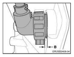
3. After installation, the correct distance between the transmission harness connector and the housing surface (B) should not exceed 3 mm.
