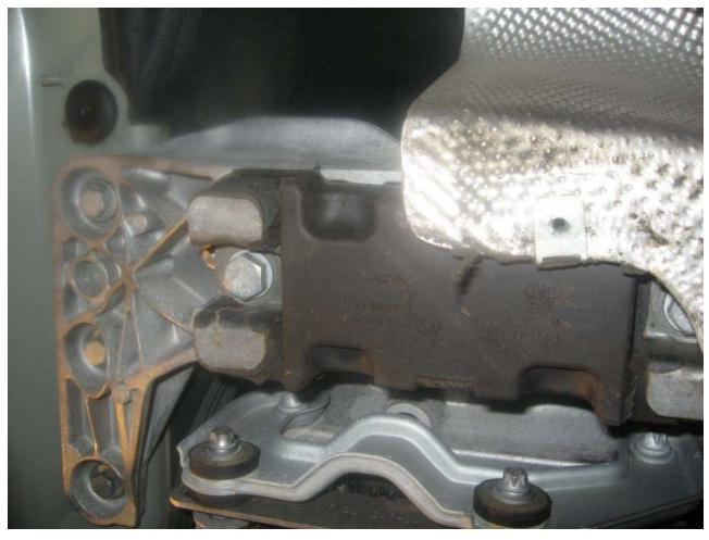
7. Remove exhaust hanger by holding E10 Torx bolt undoing the 13mm nuts. There are 3 E10 bolts plus a 4th E10 bolt between the two hangers. Once you have removed the hanger, you will have complete access to all the T-40 Torx bolts holding the transmission oil pan.
