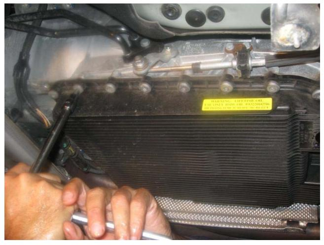
10. Drain all the fluid out of the catch can into empty container to measure. I was able to get 5.5 liters out.
