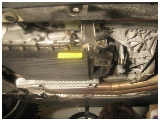
6. Remove rear transmission mount/vibration damper by undoing 16mm bolts.
