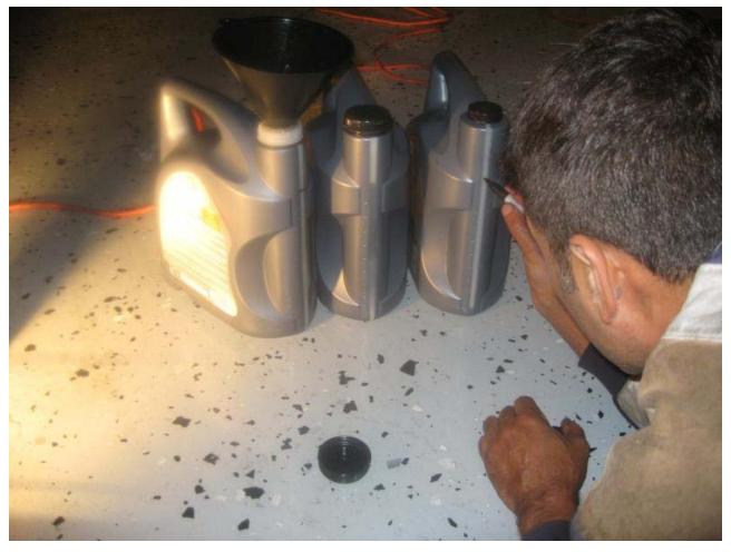
9. Once the oil stops draining, remove all T-40 Torx Bolts. Be careful to angle the pan towards the catch can because some fluid is still left in the pan. Remove pan and drain the remaining fluid in the catch can.
