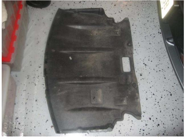
3. Remove rear under body cover using 8mm, 10mm sockets and Phillips screwdriver. This is a big piece, so proceed with care.
