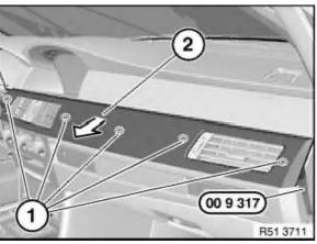
Lever out right decorative strip on instrument panel (2) at retaining points (1) with special tool 00 9 317
