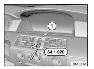
Lever out switch for hazard warning system/central locking (1) with special tool 64 1 020 and pull back.
