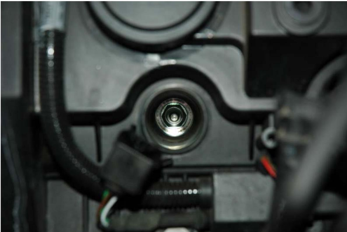
Cylinder #5 spark plug in bore
