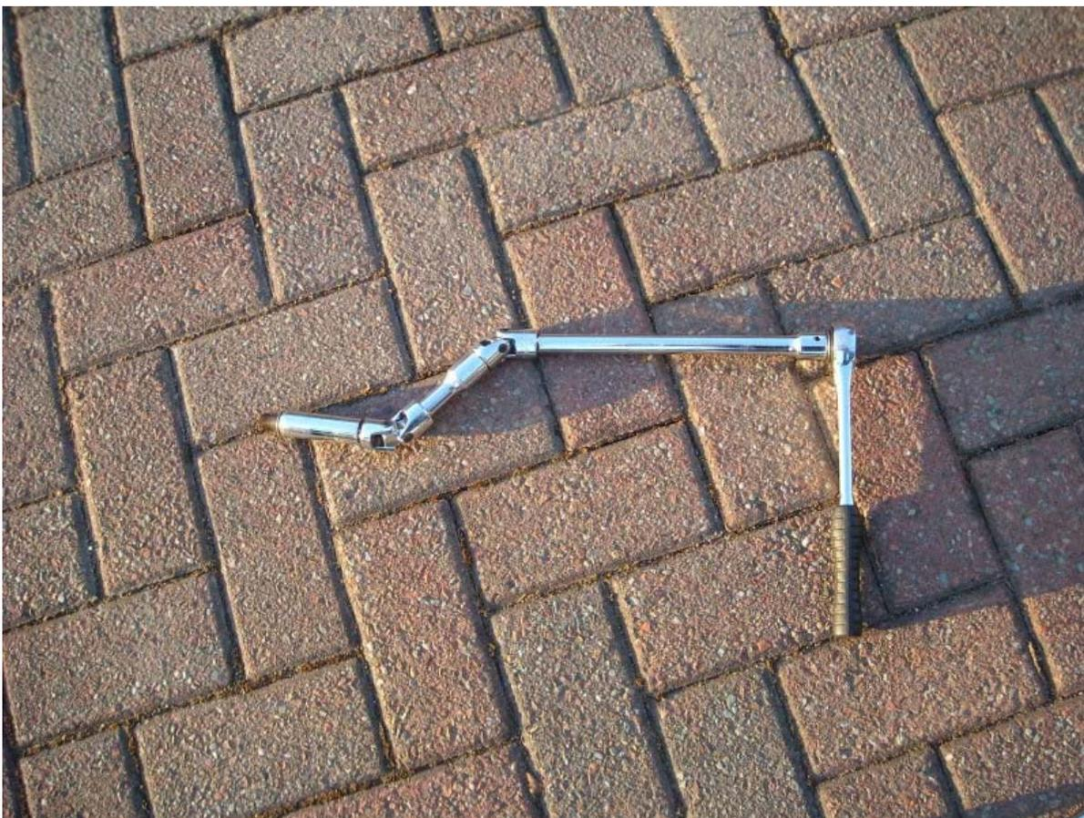
10 mm spark plug socket, universal joint, 3" extension bar, another universal joint followed by a 10" extension. This flexible arrangement could be fed into the bores quite easily.
