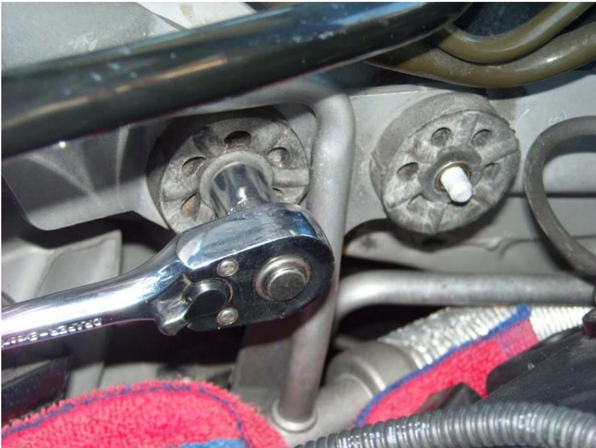
you have to remove the two 10 mm nuts that secure the air conditioning lines to the chassis rail. There are two bushes that sit over the studs to protect the rubber mounts.
