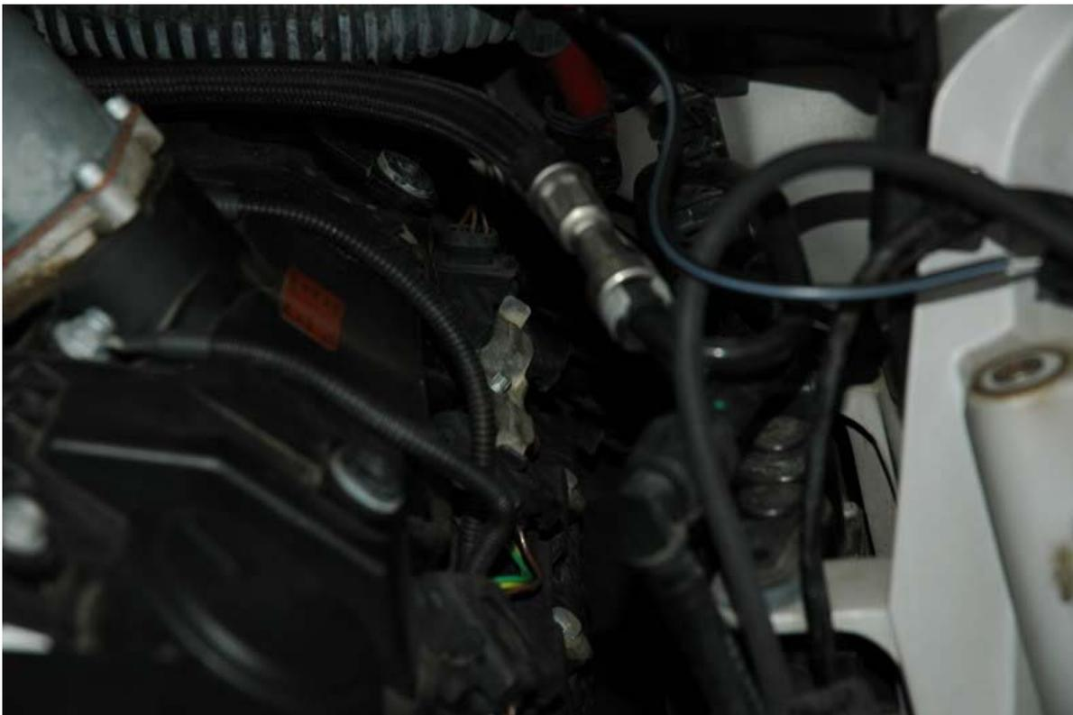
Clip retaining HT coils #7 and #8. At the bottom of the photo you can see the top of HT coil #6, I had already removed its clip.
