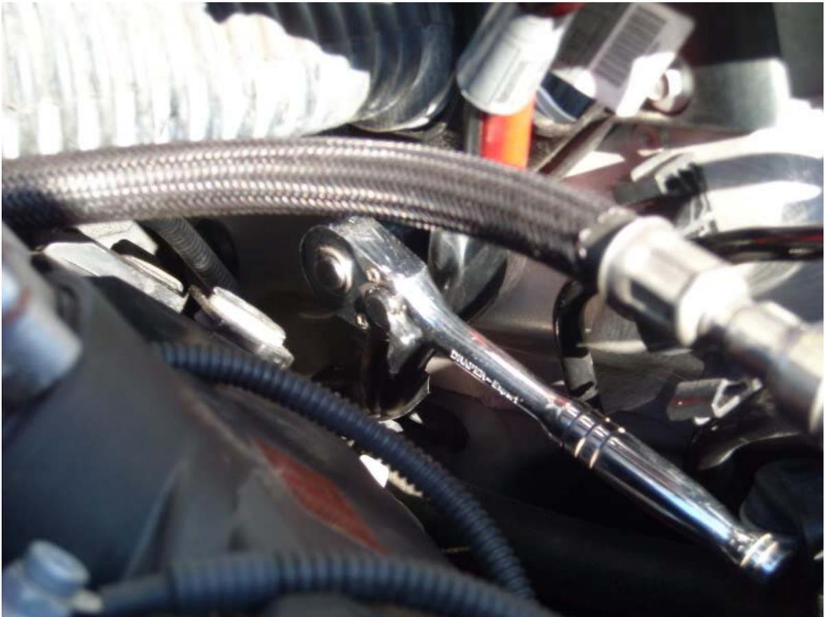
Undoing the plastic nut holding the cable housing
