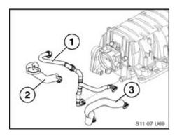
Remove the crankcase ventilation plastic corrugated hose (1) connecting the two cylinder head covers and intake system. Install the modified insulated hose with the external pressure regulating valve (2), using P/N 11 61 7 563 476. Install the insulated hose (3), using P/N 11 61 7 547 186.
