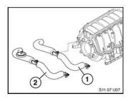
2. Remove the ventilation hose (1). Install the modified insulated hose with the external pressure regulating valve (2), using P/N 11 61 7 563 477 in the same location.
