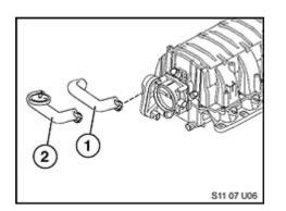
2. Remove and discard the ventilation hose (1). Install the modified insulated hose with the external pressure regulating valve (2), using P/N 11 61 7 563 476 in the same location.
