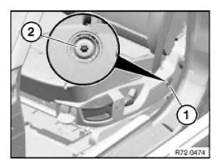
Manual/semi-electric seat adjustment only: Lever out plug (1). Release screw (2). Tightening torque 72 11 05AZ .
