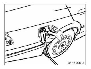
Slide extraction hose of extractor unit, refer to BMW Service Workshop Equipment and Planning Documentation, into the fuel filler pipe, turning in the process if necessary.
