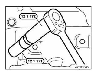
Unscrew spark plugs with special tool 12 1 171 .
