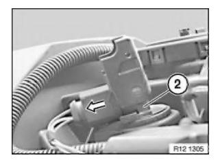
Disconnect plug. Pull out ignition coil (2). This procedure is applicable to all ignition coils.
