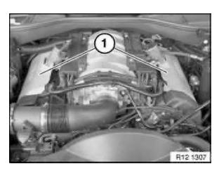
Pull ignition coil covers (1) out of rubber grommets.
