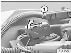
Unlock plug fastener (1) of ignition coil.
