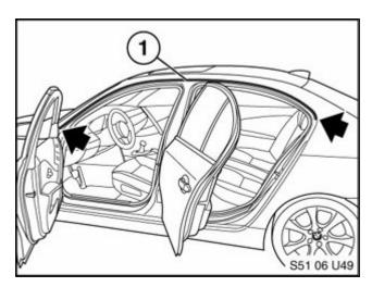
Apply a continuous length of Teflon tape
