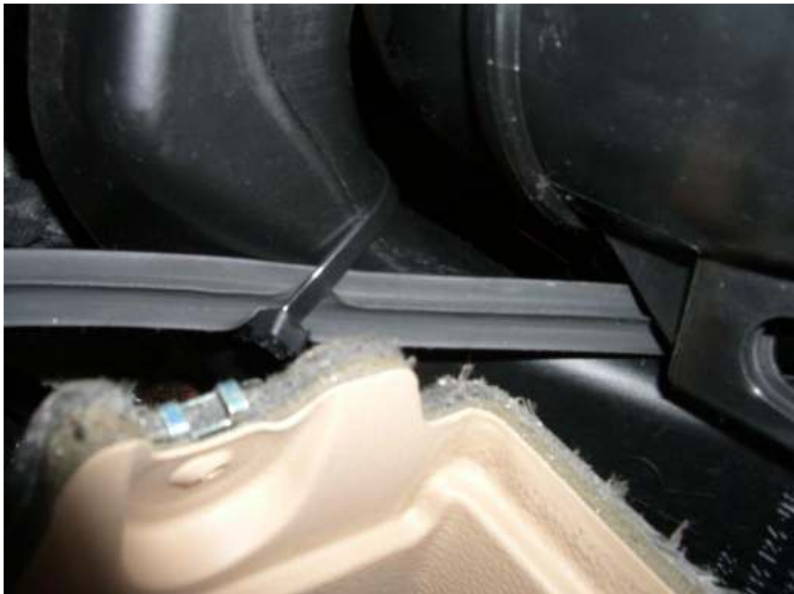
55. Right duct out. Comes out front hole better.
