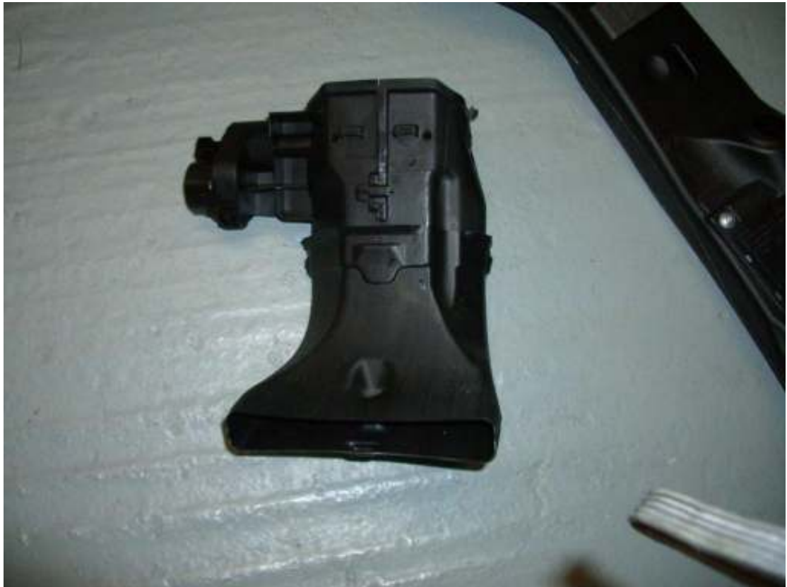
51. Left duct out. Wiggle out into the footwell.
