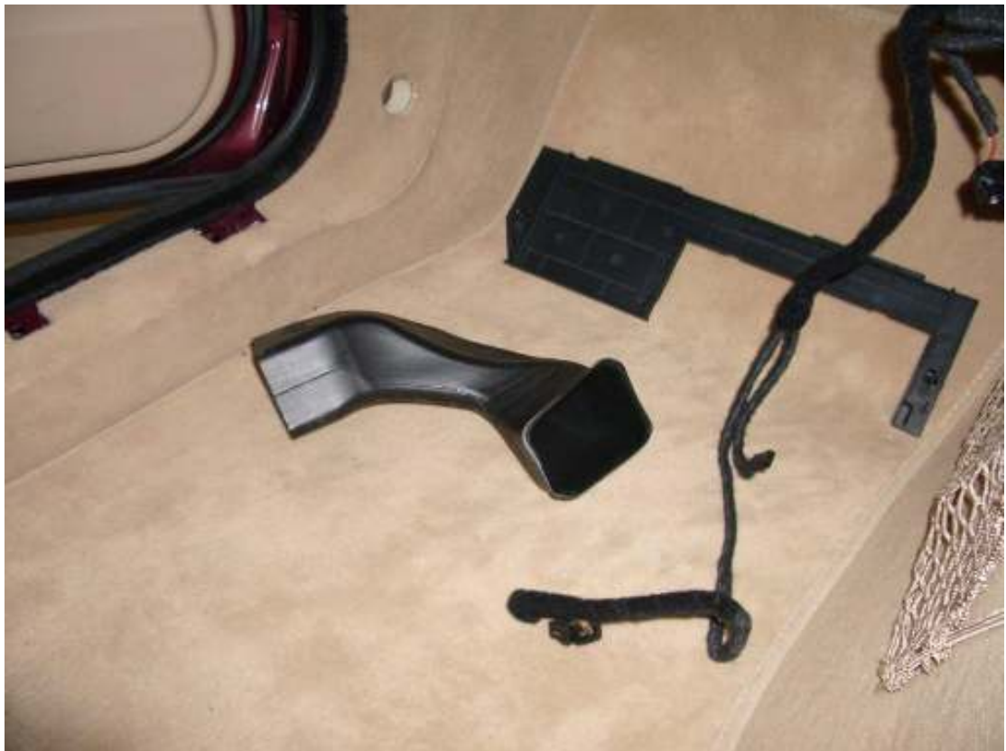
51. Left duct out. Wiggle out into the footwell.
