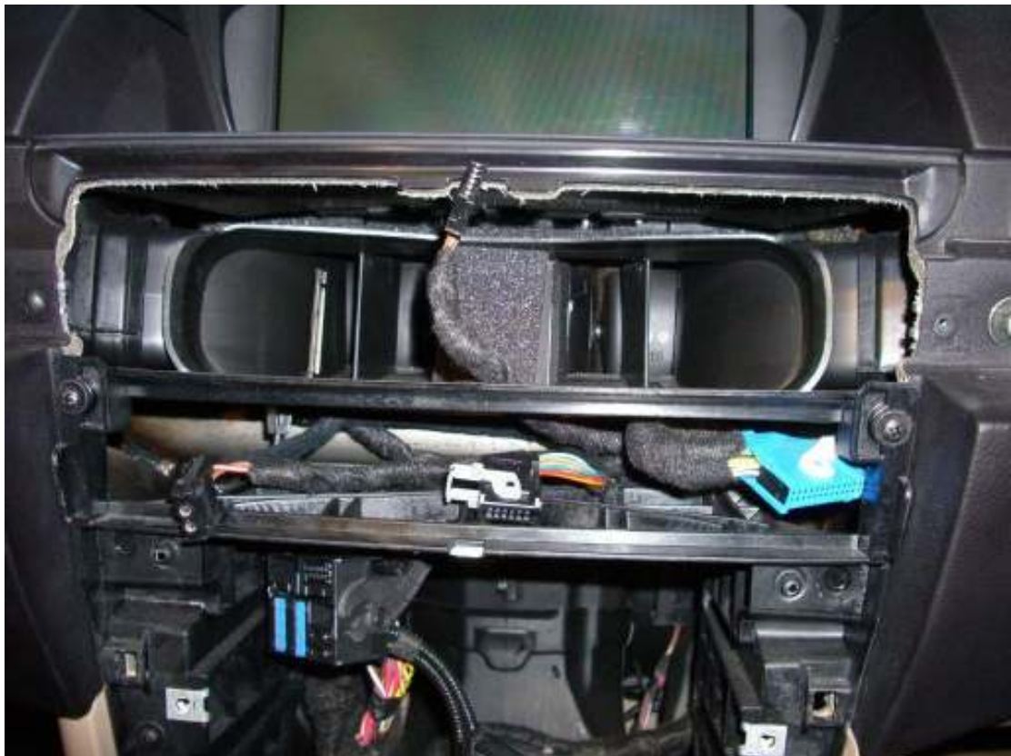
48. Central dash frame out. 6 screws. Photo the wire layout and plug positions first.
