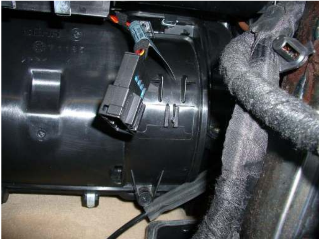
54. Cut a cable tie holding the gear selector cable to the right duct.
