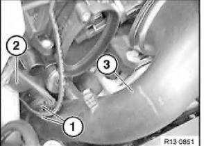
Unclip lines (1) from lower bracket. Remove hose (2). Remove intake pipe (3).
