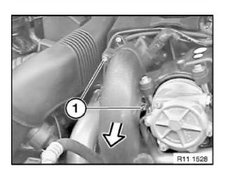
Release screws (1). Detach intake pipe a little in direction of arrow.
