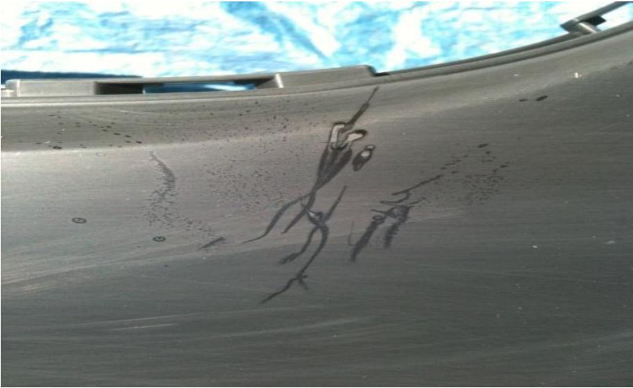
Dribble and run spots from where the cleaner came in contact with the bumper surface.
