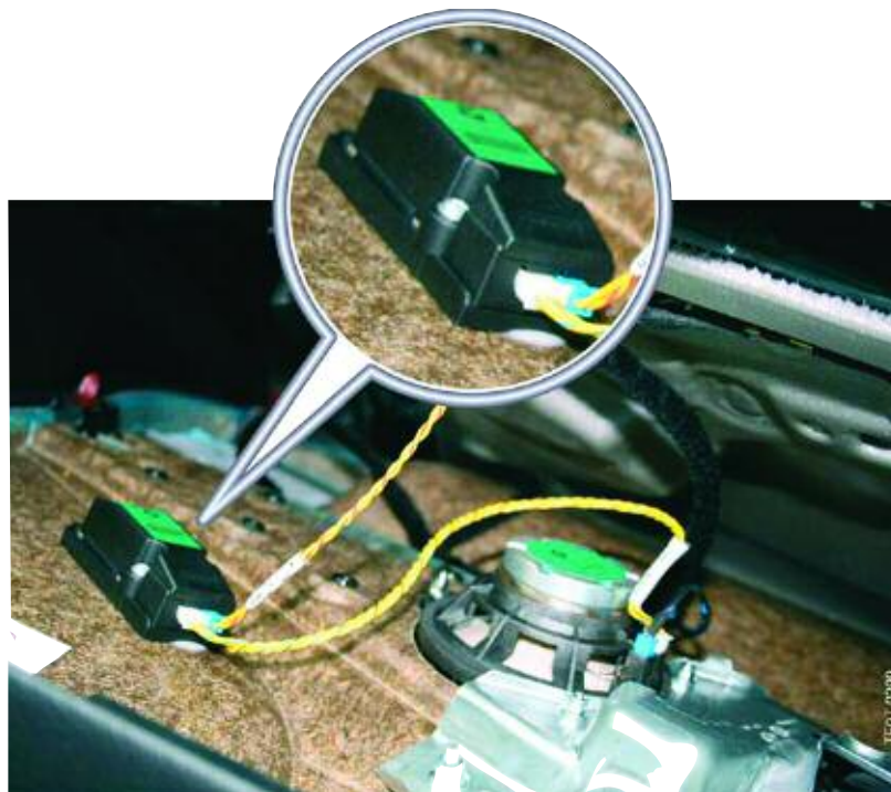
Frequency Diplexer/Crossover in the front door
