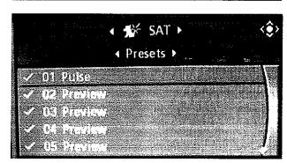
16. Store the selected satellite radio channel (e.g., channel 010 Pulse) in the "Presets" list on station 01. When stored, the station name (e.g., Pulse) will be displayed next to the station number.
