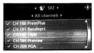
Switch to "All channels" in the "SAT" menu and select satellite radio channel 184 Preview.
