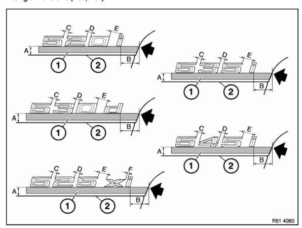
Stick on adhesive tape (1) between edge of rear lid (2) and top edge "A". Mark measurement "B" from top edge "A" to outer edge of rear lid on adhesive tape (1).
