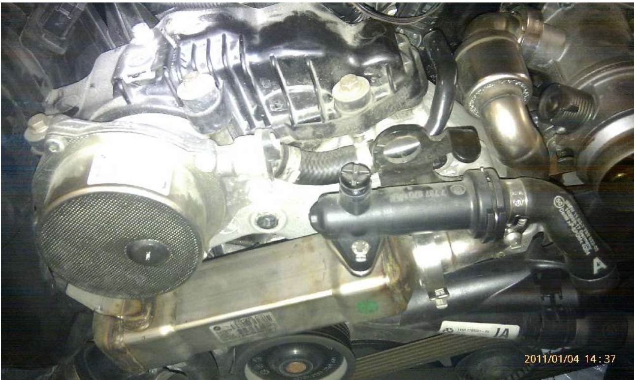
Dirty air intake. I don't know the correct name for this item, but this is where exhaust is mixed with air before entering the intake manifold. There is dirt all the way. I did not clean it this time.
