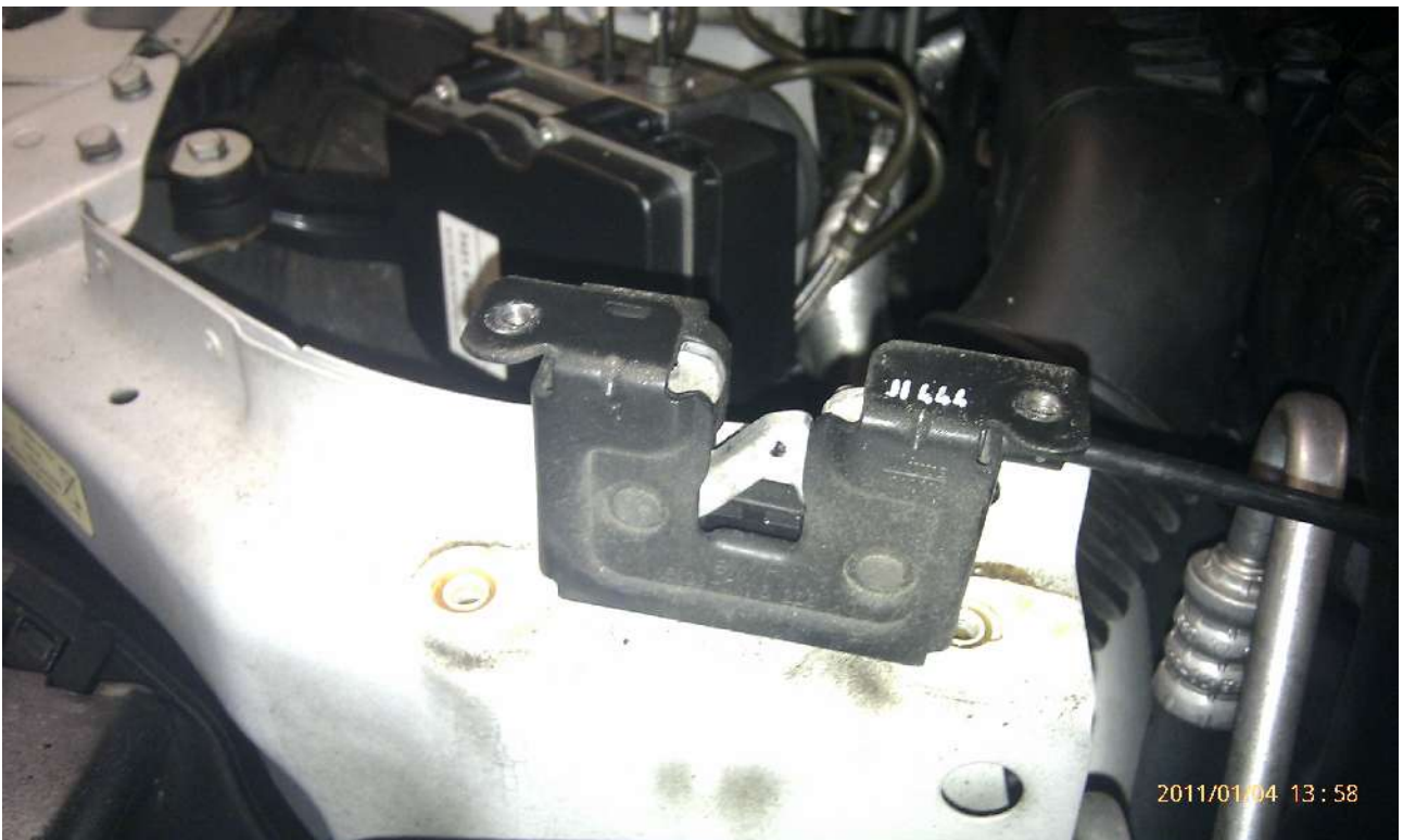
Pic showing left hood lock removed.
