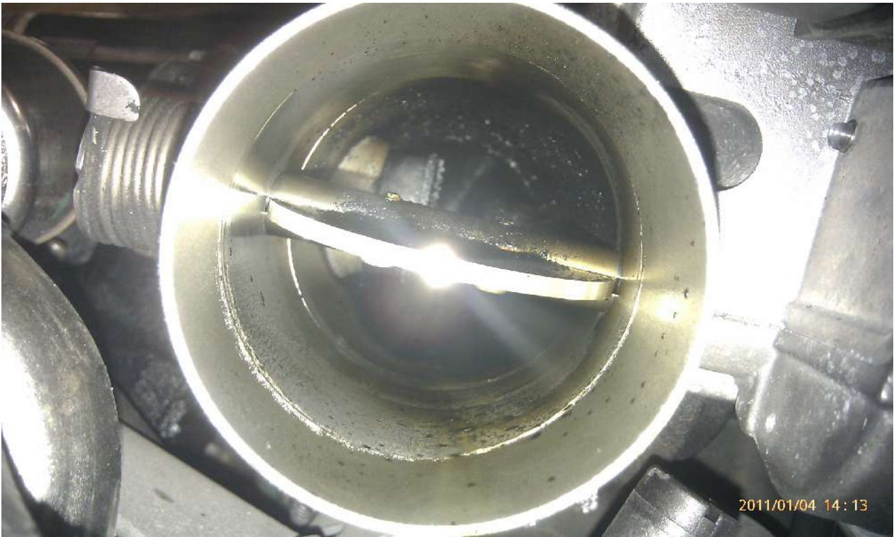
Dirty air intake. I don't know the correct name for this item, but this is where exhaust is mixed with air before entering the intake manifold. There is dirt all the way. I did not clean it this time.
