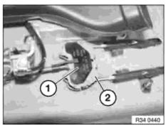
Unclip mounting clip (1) upwards out of balance arm (2).
