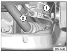
Disconnect handbrake Bowden cables at expander locks. Release screw (1) and remove bracket.
