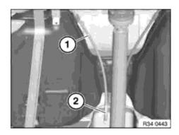
Disconnect handbrake Bowden cables (1) out of mountings.
