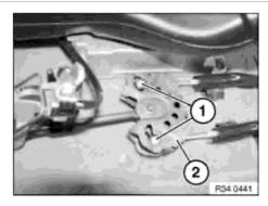
Guide handbrake Bowden cables (1) with a screwdriver inwards and pull out of balance bar (2).
