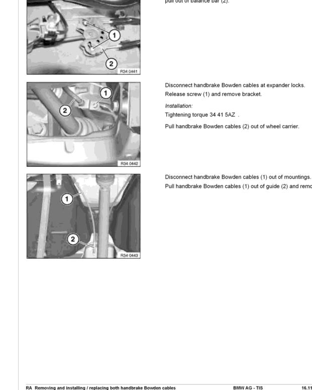
Guide handbrake Bowden cables (1) with a screwdriver inwards and pull out of balance bar (2).
