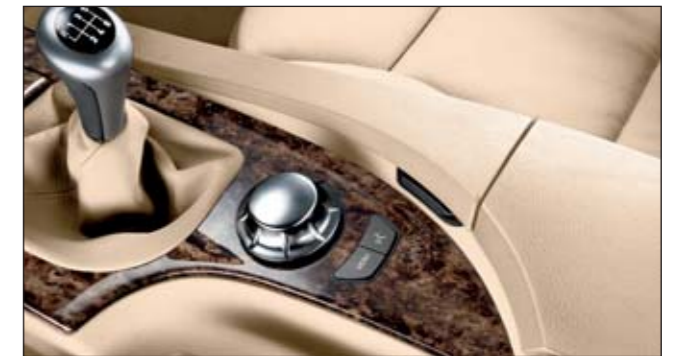
The iDrive Controller, which is conveniently located on the center console, allows you and your passenger to access and tailor many comfort features.
