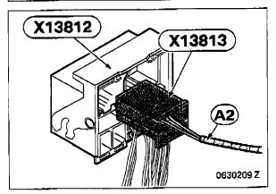
Disconnect the existing cables from branch A2 and connect them to plug X13813:
