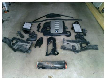
1. Remove engine cover (5 allen screws) & rubber strip
