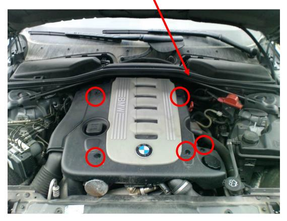
2. Remove 2x micro filters by unsnapping the hoops and turn the plastic nuts <u>one</u> <u>quarter of a turn</u> using a 13mm socket. Also remove the rubber sealings toward the fenders.
