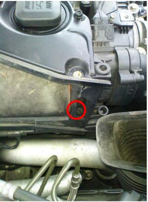
6. Remove the oil cap and lift off the filter cover. Put the oil cap back. Be amazed of the amount of debris you find inside the filter housing. Grab filter from the top side and lift it out.
