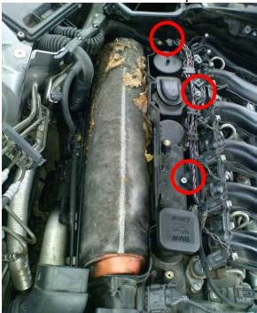
2. Loosen the 4 allen screws on the breather filter.
