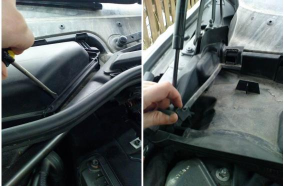
3. Remove the micro filter housings. Remove the plastic latch by lifting the circled tab and pull to the right.
