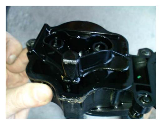
Should your filter look like the below on the other hand, you have the old type that should be changed. It's pressed in the cover so just pull it out. (pic courtesy of E60.net)
