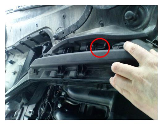
Use 13mm socket to loosen plastic nuts (3 on one side, 4 on the other) that are holding the housings. NB!! Nuts will NOT come out. They will come loose after <sup>1</sup>/<sub>4</sub> turn.
