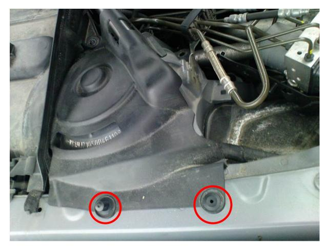
Remove the strut brace. 4 x T45.
