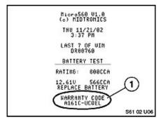
On completion of a battery test, print out the results, and file the printout with the completed repair order for future reference, if requested.
