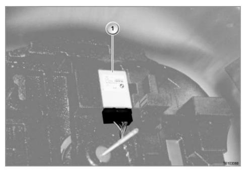
A 15-pin connector links the MPM to the vehicle electrical system and the K-CAN. The K-CAN connection allows the exchange of CAN messages between the control units of the body electronics.
