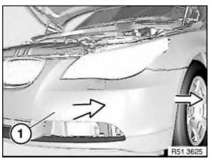
Press bumper trim (1) against direction of travel and release from side holders in direction of arrow.
