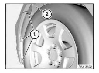
Release screws (1) on wheel arch trim (2) on left/right.
