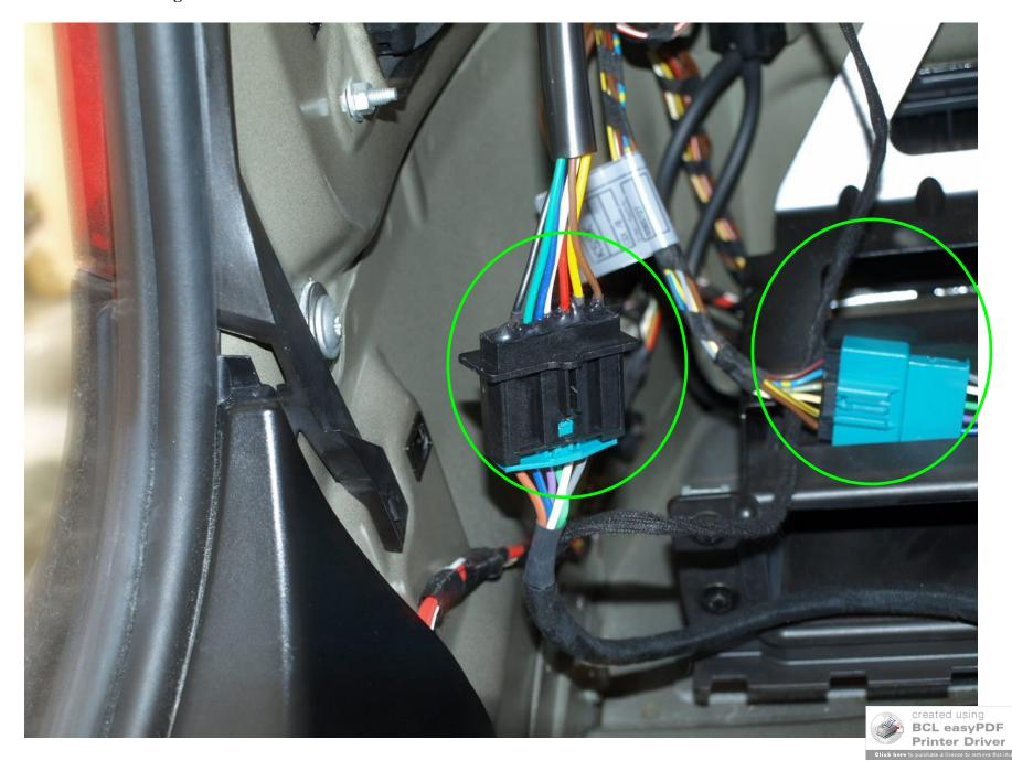
6. Now, mount the cable module by unscrewing the screw located under the tail light.
