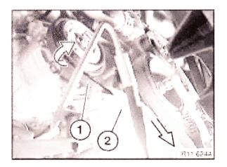
Rotate engine at central bolt in direction of engine rotation.
