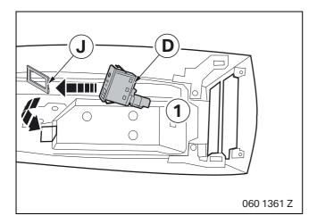
Clip the USB/AUX-IN socket holder **J** to the location of the previously-removed ventilation nozzle in the oddments box of the centre console (1).
