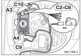
On cars with **SA 620** and without **SA 609**, the High charger/hands-free electronic module is already installed. ◀
