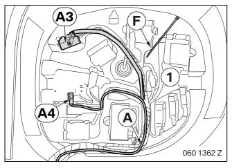
Route branches **A3** (black 54-pin socket casing) and **A4** (HSD socket casing) into the oddments box (1).
