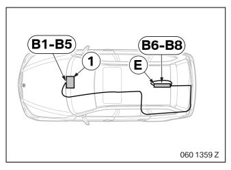
Route branch **B1–B5** to the installation point of the CCC/M-ASK (1).
