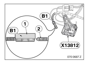
Release the fibre optic cable connector (1) of branch **B1** and connect the previously disconnected fibre optic cable (2).
