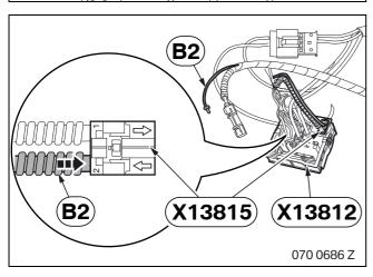
Unclip fibre optic cable casing **X13815** (SW 2-pin) from plug **X13182** (SW 16-pin).
