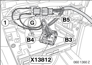
Disconnect the cable (1) from plug **X13812** (black 16-pin) and connect to socket casing **G** as follows:
