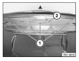
Version with rear window roller blind only: Release screws in luggage compartment.
