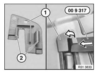
If necessary, remove or replace rear window roller blind:
