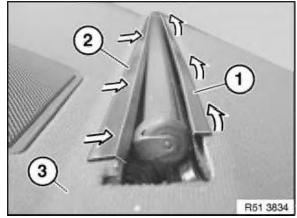
Lift out shelf (3) over rear groove (1) of rear window roller blind. Pull front guide (2) out of shelf (3) and remove roller sun blind towards bottom.
