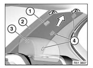
Lever out airbag emblem (1) and release screw underneath.
