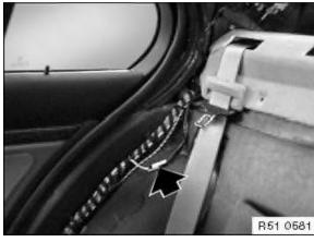
Version with rear window roller blind only: Disconnect plug connection (1).
