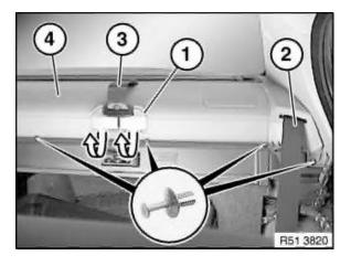
Release center seatbelt finisher strip (1) and feed out seatbelt strap (3).
