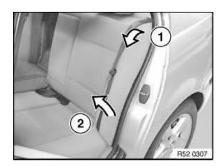
Pull seat belt to middle and place behind head restraint.
