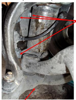
I would guess the black wire is the ABS sensor. Use 5mm allen to remove it. In this pic you can also see 3 of the 4 18mm bolts holding the bearing. The 2 to the left you can reach without problem so remove them. The lower one was a real pain to get out due to the loctite and I had to add an extension pipe to get enough torque.
