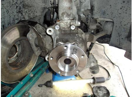
When putting the shock back in place, note that there is a notch on is that needs to go in the clamping slot on the backside. Clamp shock, assemble ABS sensor, sway bar rod bracket and you're done!! Reassemble the brakes and wheel and enjoy the silky smooth drive.
