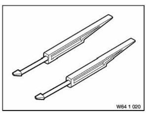
Note: For releasing and removing fresh air grilles -
