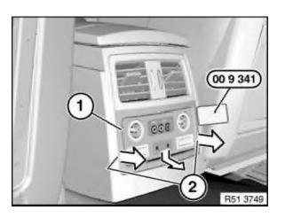
Unclip rear insert (1) with special tool 00 9 341 at retaining points (2) and pull back in direction of arrow.
