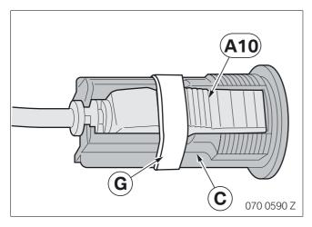
Secure branch A10 in USB holder C with cable tie G.
