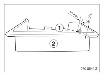
Drill a hole (1) on the glovebox insert (2) at the dimensions shown and drill through using a 25 mm step drill bit.
