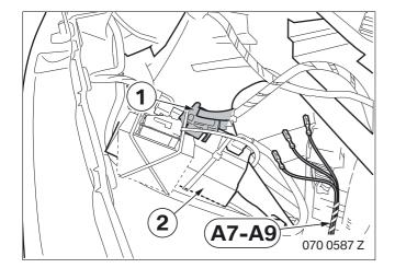
Disconnect branch (1), BL 26-pin socket casing (branch **A15** of the ACM wiring harness) from the ACM unit and unlock.
