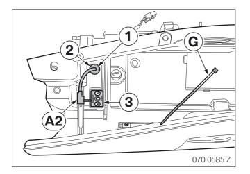
The depiction is an example. The hole must be drilled specifically according the type of car or customer's wish in the vicinity of the AUX socket (3).
