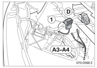
Connect branches **A3-A4** as follows to socket casing **D**:
