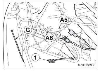
Connect branch (1), SW 3-pin socket casing (branch **A20** of the ACM wiring harness) to branch **A5**, SW 3-pin plug casing.
