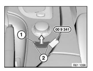
Unclip button unit (1) with special tool 00 9 341 at retaining points (2) and lever out in direction of arrow.
