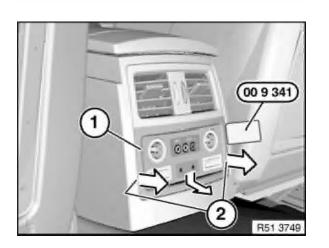
Unclip rear insert (1) with special tool 00 9 341 at retaining points (2) and pull back in direction of arrow.
