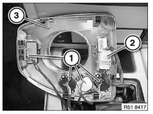
Reach into trim (1) and unclip upwards from retainers (2).
