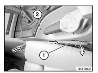
Lever out trims (1) on left/right at rear end and pull out of storage compartment in direction of arrow.
