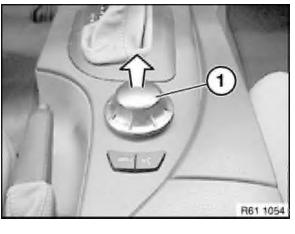
Detach knob for controller (1) in direction of arrow.
