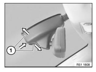
Detach two-part mirror base cover (1) by pressing from below. Feed out two-part mirror base cover (1) and remove.
