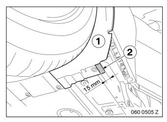
Separate the marked section (2) from the wheelhouse liner (1).
