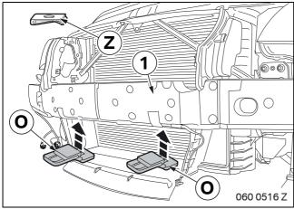
Screw adapter **O** onto the middle two attachment points of the bumper trim on the bumper support (1).
