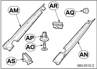
Insert clips **AR** and **AS** into side member trims **AM** and **AN**.
