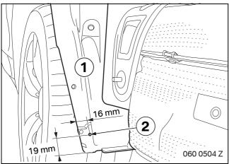
Drill an 8 mm hole (2) in the wheelhouse liner (1) using the dimensions shown.
