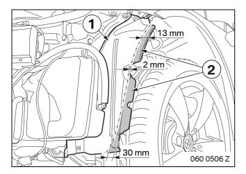
Separate the marked section (2) from the wheelhouse liner (1).
