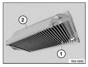
Lever microfilter for interior ventilation (1) in direction of arrow out of microfilter air duct (2) and remove.
