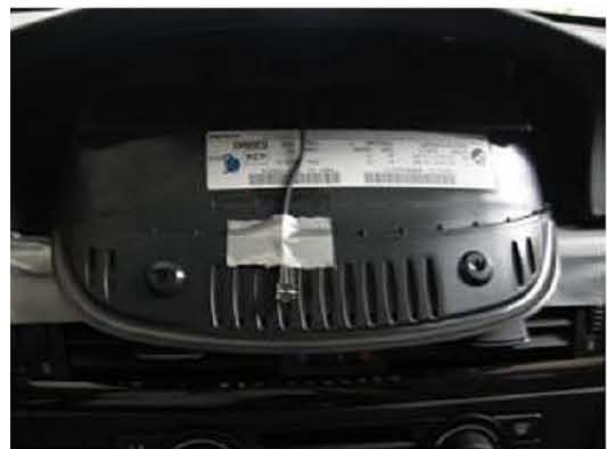
STEP 14: Secure the remote eye in a location that it will receive the Remote signal
