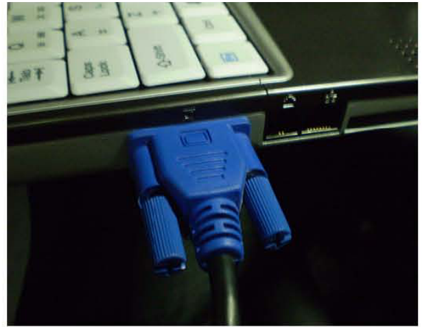
STEP 11: Connect VGA Cable to CAR-PC Make sure that this connection is secure.
