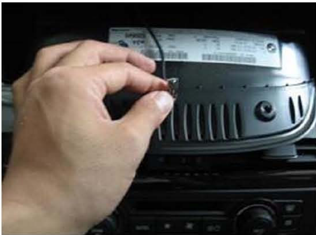
STEP 13: Run the wire for the remote eye so that the eye can line up with the remote signal.
