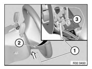
Insert T25/T27 Torx screwdriver (1) from below into hole (2) until a springy resistance can be felt through annular spring (3) of airbag unit. Continue to press in T25/T27 Torx screwdriver (1) until airbag unit is released.
