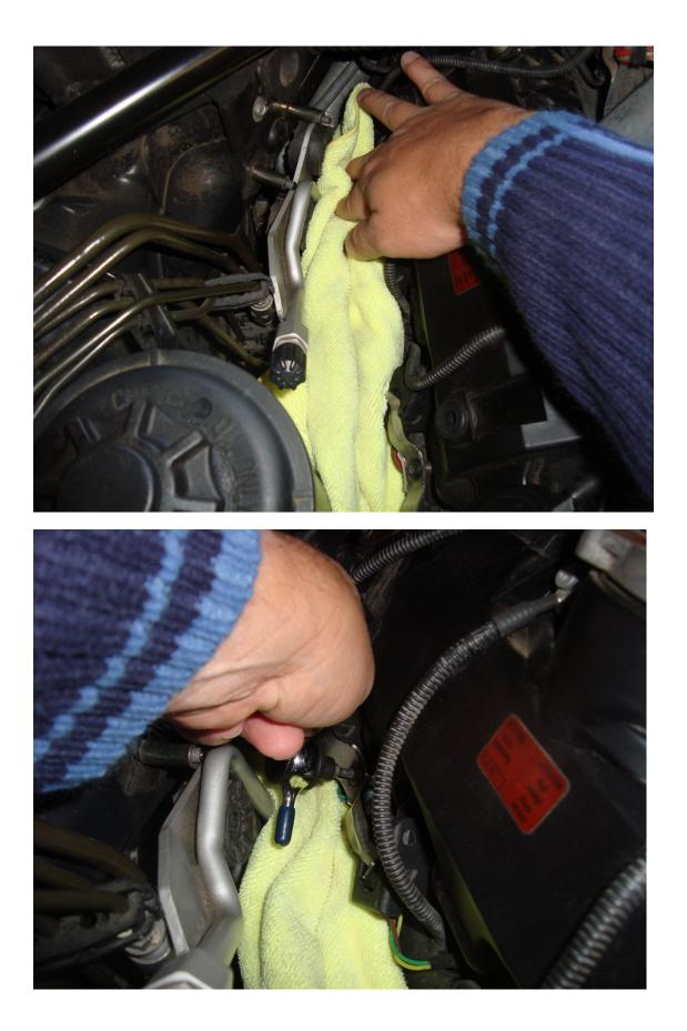
Fifth Step: that is it..... Now you can replace the spark plug #4 easily now.... Just remove the ignition coil.
