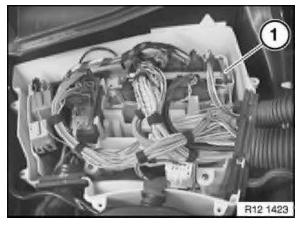
Unlock and detach all plug connections on DME control unit (1). Unlock DME control unit (1) and remove towards top.
