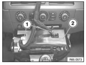
Unlock plug connections (1) and disconnect.
