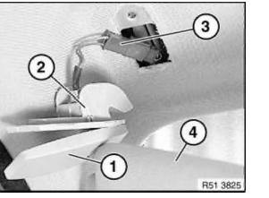
Lift out sun visor. Pull out cable slightly and disconnect plug (3).
