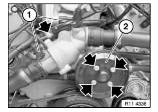
Unlock and detach plug connections (1).
