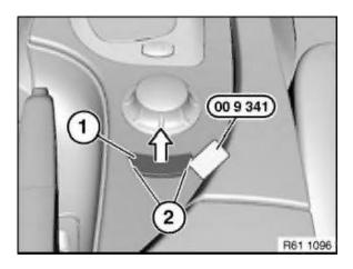
Unclip button unit (1) with special tool at retaining points (2) and lever out in direction of arrow.
