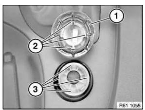
Detach knob for controller (1) in direction of arrow.
