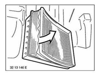
Remove air cleaner element from intake filter housing.
