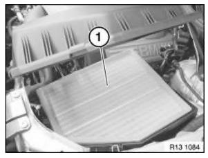
Open clips (1). Lift top section (2) of intake filter housing.
